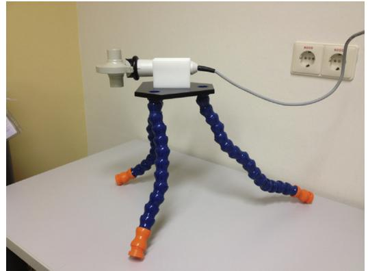
**Fig. 13.** MR-imaging-compatible spirometer. Mouthpiece of an MR-imaging-compatible spirometer is standing on a plastic tripod within the MR imaging suite.
